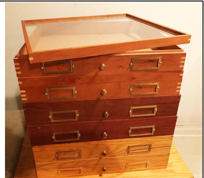
Cornell drawers (6): Custom built of fine hardwood. 2 each of cherry, red oak, and mahogany. Corners are mitered and splined, hardboard bottom set in slots for strength with glass tops. Pulls and 2 card holders. $300 for all 6.
